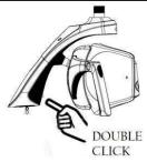
Every time a double click is performed, the Tk of the light changes. Repeat the procedure until the desired colour temperature is shown on the indicator light. 2 beeps will inform the user that Tk is changing.
