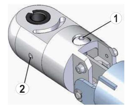
Secure the 3 grub screws (2) with safety lacquer (blue).
