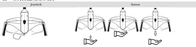
Push right or left and release Acoustic signal: I beep
