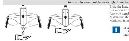
Bring the hand towards the sensor up to 2 cm and keep this distance until the desired light intensity is reached Acoustic signal: 1 beep at command Maximum intensity reached: 2 beeps Minimum intensity reached: 1 beep
